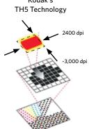
Thermal (25 watts) 128 channels Tonal stability – medium to HIGH Exposure uniformity – HIGH
